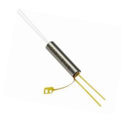
The mini MEMS Variable Optical Attenuator Integrated with Input Optical Power Monitor is a hybrid fiber optical device that integrates a thin-film tap of flat spectral response and a high sensitivity PIN photodiode for power monitoring applications with a MEMS VOA. The Power Monitor minimizes component assembly costs and module footprint. The thermal MEMS VOA has little temperature dependence and drift. It is intrinsically more reliable than electrostatic MEMS VOAs.
